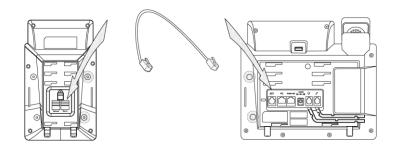
If you connect two expansion modules, connect the Ext out jack of the previous expansion module and the Ext in jack of the second expansion module using another supplied cord.
