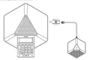
Note: Up to two expansion microphones can be connected to an IP conference phone.
