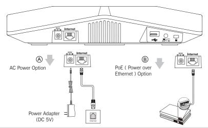
Note: The IP phone shoule be used with Yealink original power adapter (5V/2A) only. If inline power (PoE) is provided, you don't need to connect the power adaper. Make sure the hub/switch is PoE-compliant.
